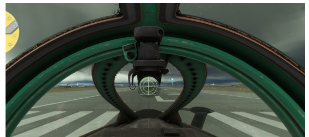
MiG-25PD close-range optical gunsight (Pic. 4)
