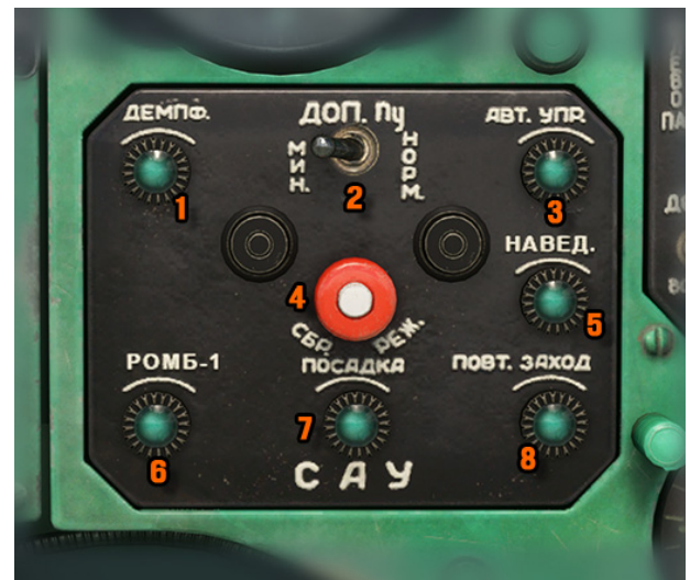
SAU (Automatic Control System)
