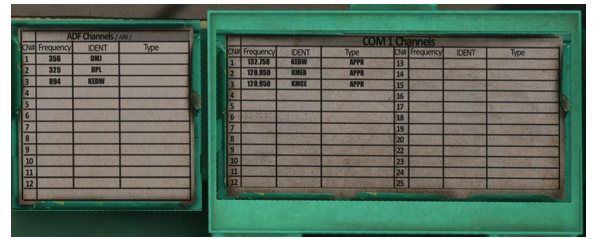
ADF and COM Channel Cards (Pic. 8)
