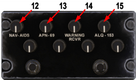
TYPICAL AUXILIARY MIXER SWITCHES FOR THE PILOT, COPILOT, INSTRUCTOR PILOT, RADAR NAVIGATOR, NAVIGATOR, INSTRUCTOR NAVIGATOR, EW OFFICER, DEFENSE INSTRUCTOR, AND GUNNER
