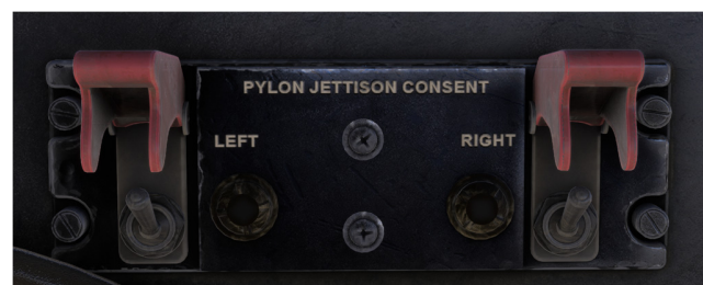
Figure 2-05. PYLON JETTISON CONSENT panel.
